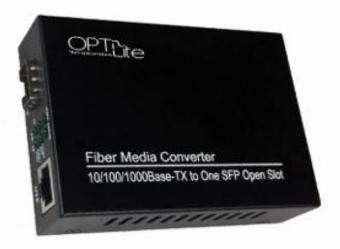
This is an intelligent, adaptive and efficient Ethernet converter device. It can implement data transmission between twisted pair electrical signals and optical signals, which are the two types of network connection media. This type of media converter can extend the transmission distance to 0.55 kilometres (multimode) or 120 kilometres (single mode). Using a media converter is an economical solution to achieve a long distance transmission, based on current status.
