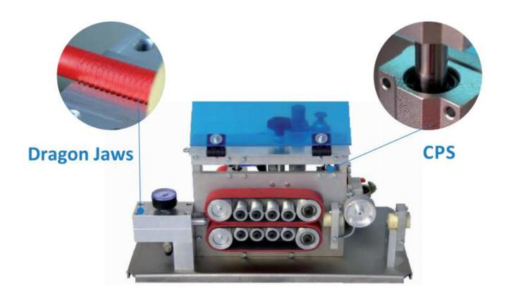
This professional micro cable blower designed for blowing micro cables with the diameter from 4 to 10 mm is new on the European market. Micro Cable diameter from 5 to 16 mm. Solid and simple construction enables easy operation of the blower and long-term durability. Due to high quality of the tray and power of the pneumatic engines the blow speed of up to 110m/min is available at a distance up to 2,5km. The distance of up to 3,5km is possible when we use water instead of air.
