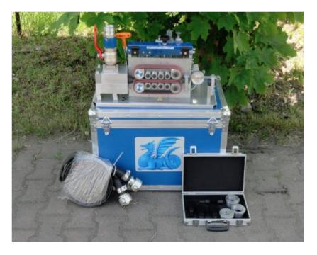
This professional cable blowing machine is designed for blowing cables with the diameter from 6 to 15 mm. Ducts diameter 32mm, 40mm and optional 50mm. Solid and simple construction ensures ease of operating the machine and allows to preserve the reliability. High quality feeder and power of pneumatic motors allows to blowing cable with the speed up to 110m/min and for distance up to 2,5km.
