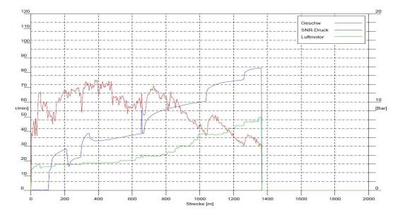
The blue line in the diagram shows the correct way to pressurize the microduct
